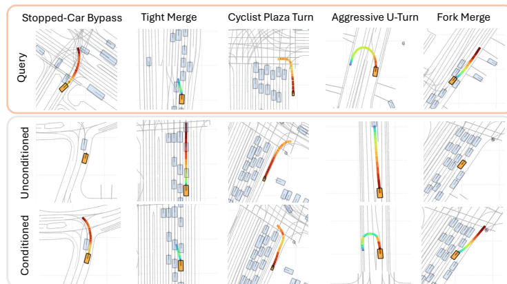
Fig. 6: Qualitative results of long-tail scenario generation. Top: Source scenarios providing the target long-tail behavioral latents. Middle: Default base model predictions in the retrieved matching contexts, showing only nominal driving. Bottom: Our framework successfully injects the queried intent, enabling agents to execute complex, safety-critical maneuvers realistically in novel contexts.
